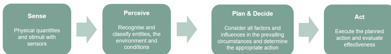
Figure 3: High level functional flow diagram for ASV decision making
